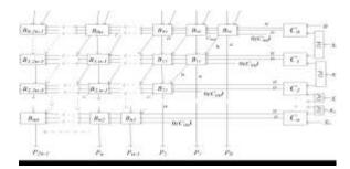
**Theorem 1:** Let NGT be the number of gates required to realize an  $n \times n$  Reversible Multiplier where n is the number of bits, then  $NGT \ge 9 \ 2 \ n2 + 1$  (5)
